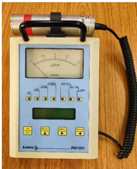
Figure 1. RM1001-RD LAMSE survey meter calibrated from SSDL Pakistan
